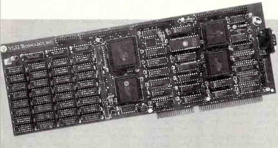
**A glimpse of goodies to come — an add-in card for an IBM PC/AT or close compatible with which you can explore RISC technology without breaking the bank or burning your brain cells.**
