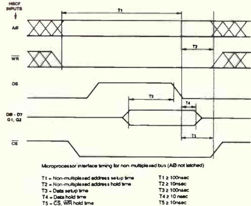
Figure 12. Timing diagram for non-multiplexed bus.
