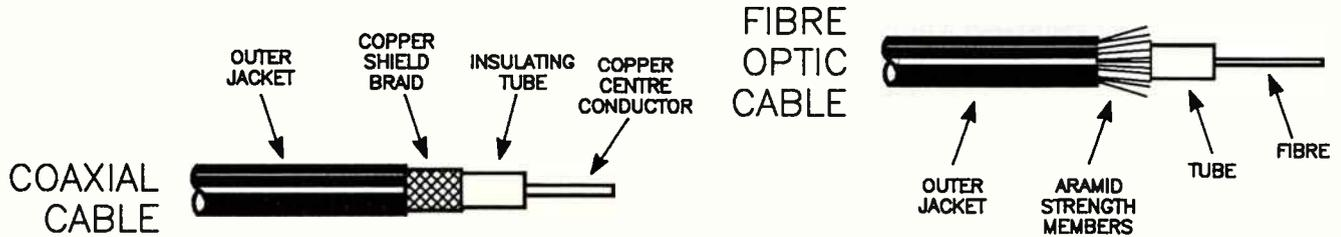
Illustrating the differences between the construction of coaxial cable and today's fibre optic cable.
