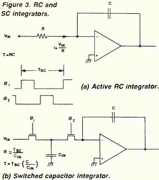
two-phase, non-overlapping clocks:  $\phi_1$  and  $\phi_2$ . The period of these clock signals is  $T_{SC}$ .
