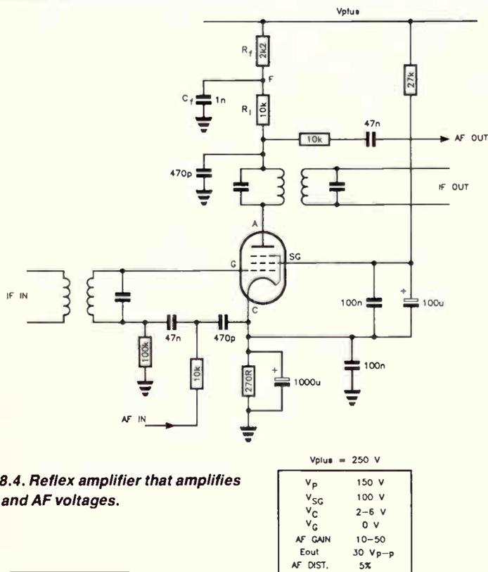
Figure 8.4. Reflex amplifier that amplifies both IF and AF voltages.
