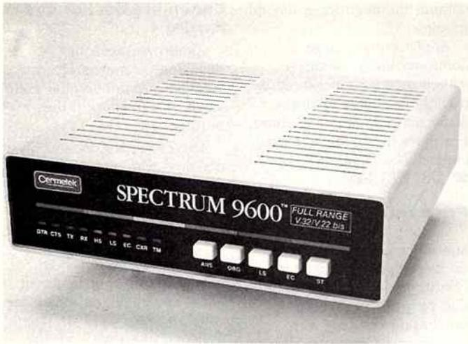
incorporates 'smart' software that automatically switches from leased line operation to an alternate PSTN line in the event of a failure. The whole process is transparent to users.
