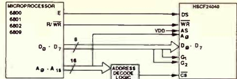
Figure 11. Motorola 8-bit bus connection.
