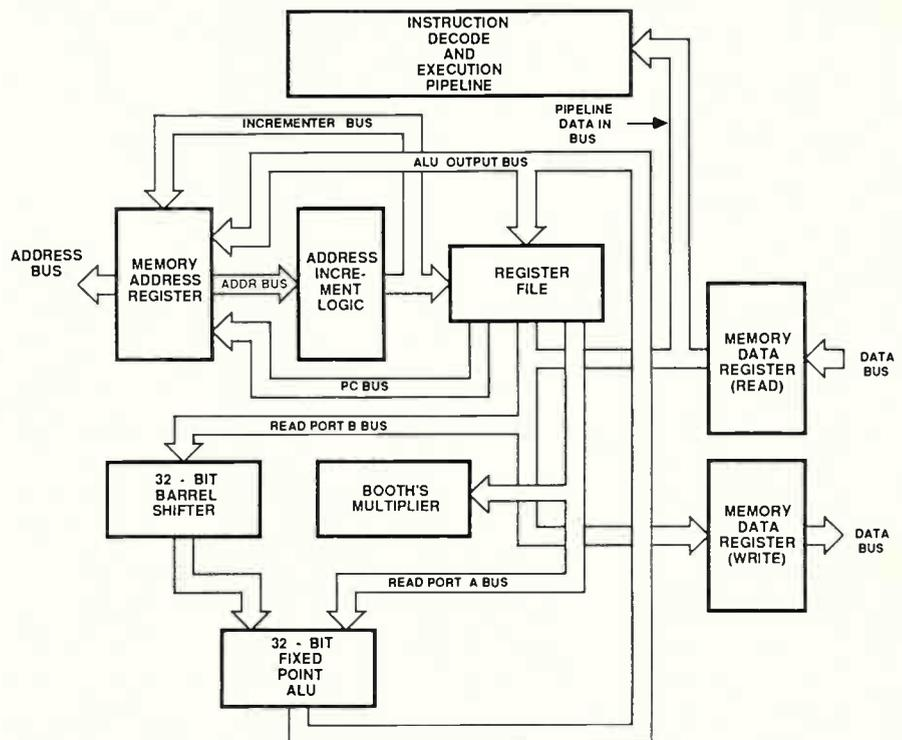
**Figure 5. Block diagram of the VLSI VL86CO10, a low cost RISC processor.**
