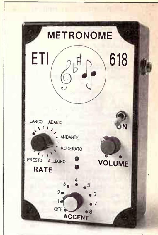
The metronome is housed in an all-plastic jiffy box, with the front panel dressed up with a Dynamark escutcheon.
