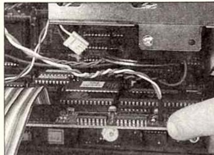
**7** One flying lead you may not have been able to connect, depending on whether or not you have a hard disk, is the connection for the hard disk operation indicator. This attaches to the hard disk controller card and so can only be connected once this is installed.
