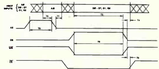
Figure 15. Timing diagram for multiplexed bus.
