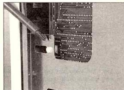
**1** As can be seen in the picture the case provides for the mounting of the main computer board using copper and nylon
