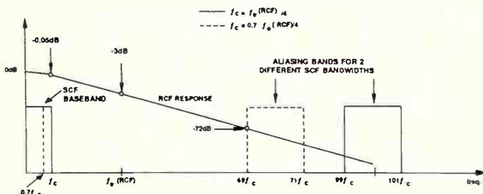
Figure 17. Alias damping from RC filter.
