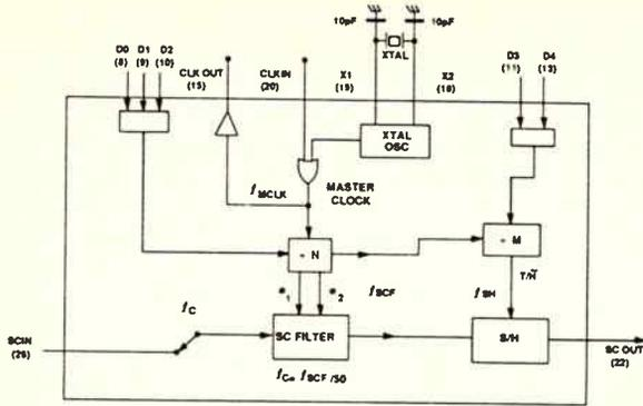
Figure 5. HSCF24040 Partial block diagram.
