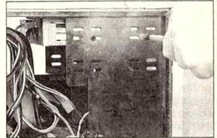
**9** Once the drive is in position, four screws are needed to secure the drive to the case. I have noticed in doing the three different installations that the types of screws needed to do this vary from drive to drive. If there are no suitable screws in the hardware supplied with the new case you should use the screws left over from your old system.
