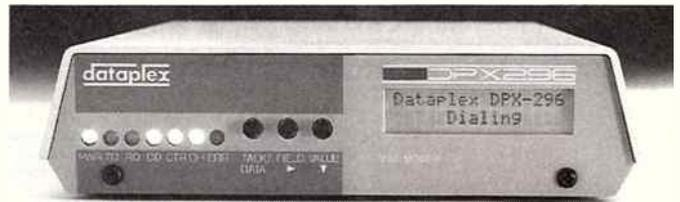
modem's front panel, allowing entry of phone numbers and communications parameters. Dialling of up to 20 stored telephone numbers can be accomplished by selecting the numbers from the front panel display.
