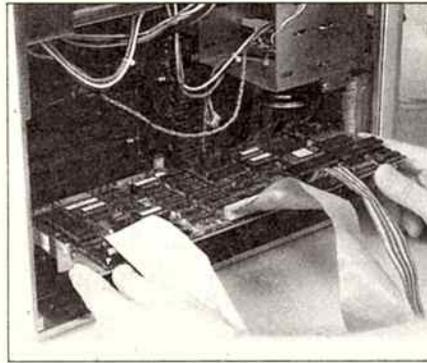
**6** Re-installing the add-on cards is the next step, after checking all flying leads are properly connected. This is a simple matter of sliding the card into an appropriate slot and 'rocking' the card slightly in order to secure it in the edge connector on the motherboard. Be careful not to put too much pressure on the motherboard as it may flex the board to a point where it cracks, or breaks a track.
