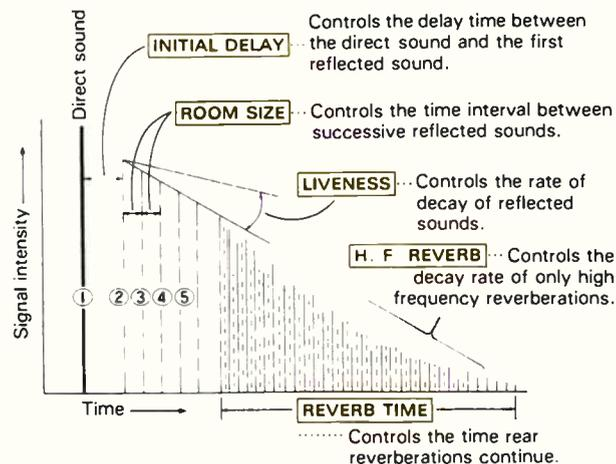
**By changing the parameters of a preset program, you can create different sound fields. The six parameters are: 1) Initial delay; 2) Room size; 3) Liveness; 4) Reverb time; 5) HF reverb and 6) P front EQ, rear EQ.**
