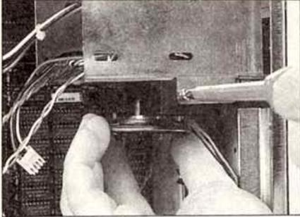
**4** The speaker and its mounting hardware are then secured, using a self tapping screw, to the plate of metal protruding from the underside of the drive enclosure inside the case.
