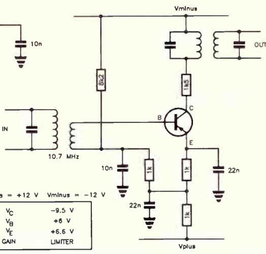
Figure 8.2. PNP transistor RF/IF limiting amplifier.
