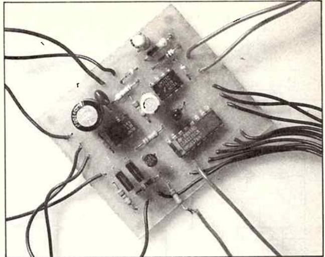
important; get one or more wrong and it won't work, apart from the possibility of damaging an IC, for instance. Note that the 4017 (IC2) is a CMOS type and, while it features protected inputs, follow the usual precautions for handling CMOS: only pick it up by the ends and avoid touching the pins. Solder its ground (pin 8) and supply (pin 16) pins before the others.
