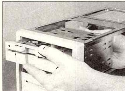
**8** Next step is to mount the drives in their enclosure, starting with the floppy disk drive. The first part to mounting the floppy drive,
