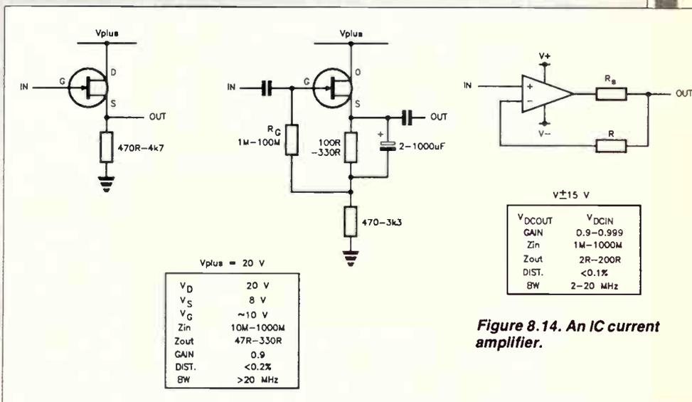
Figure 8.14. An IC current amplifier.
