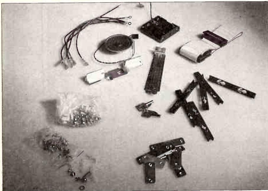
Your case will be supplied with a "hardware" kit, containing screws, pc board spacers, battery holder, slot brackets, blanking panels, slot guides and other paraphernalia.
