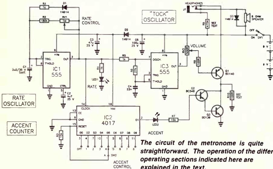
The circuit of the metronome is quite straightforward. The operation of the different operating sections indicated here are explained in the text.
