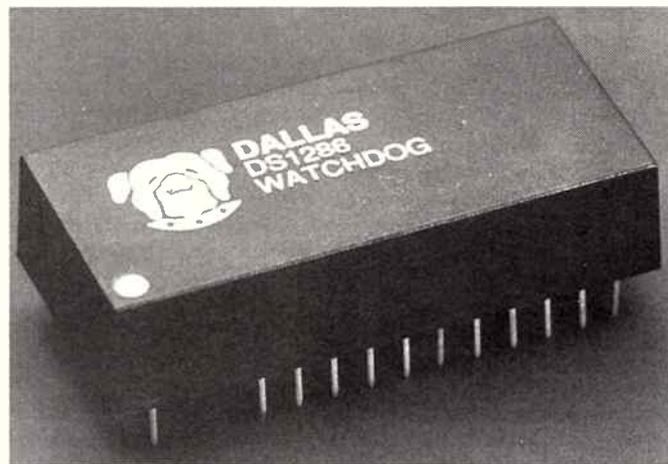
THE DS1286 Watchdog Timekeeper from Dallas Semiconductor keeps track of time with its 400-year calendar and features a watchdog timer that guards against computer malfunction.
