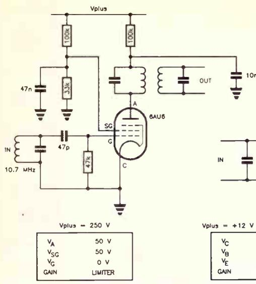
Figure 8.1. Valve RF/IF limiting amplifier.
