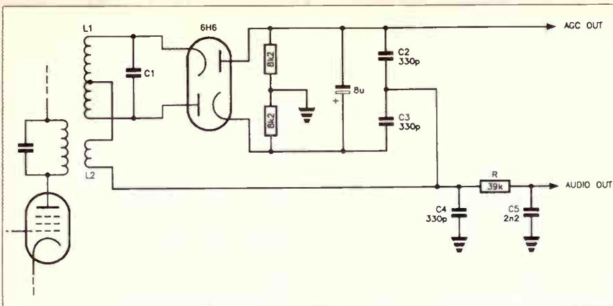
Figure 8.9. FM ratio detector.
