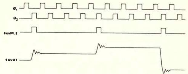
Figure 7. S/H sampled SC filter output.
